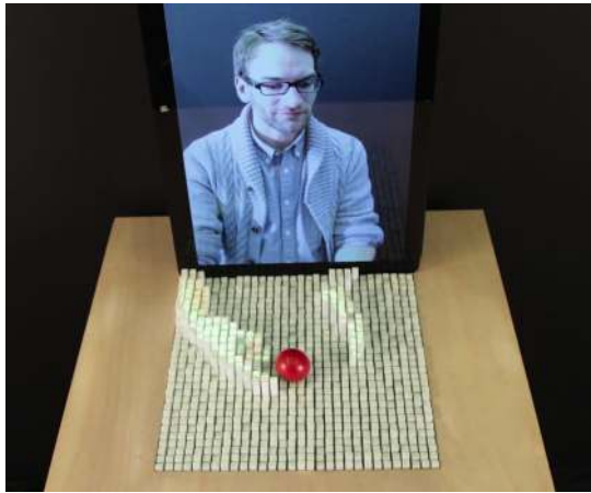
Figure 2. A user manipulating a sphere through his remote physical embodiment.
