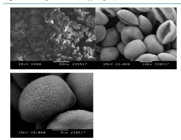
Figure 2. Scanning Electron Microscopy Images of Date Palm Pollen
