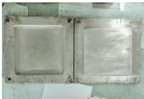
Figure 1. Picture of the die that was used to prepare the composites.
