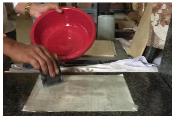
Figure 3. Hand lay-up technique for fabrication of composite laminate.
