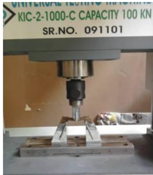
Figure 6. Experimental flexural test specimen.
