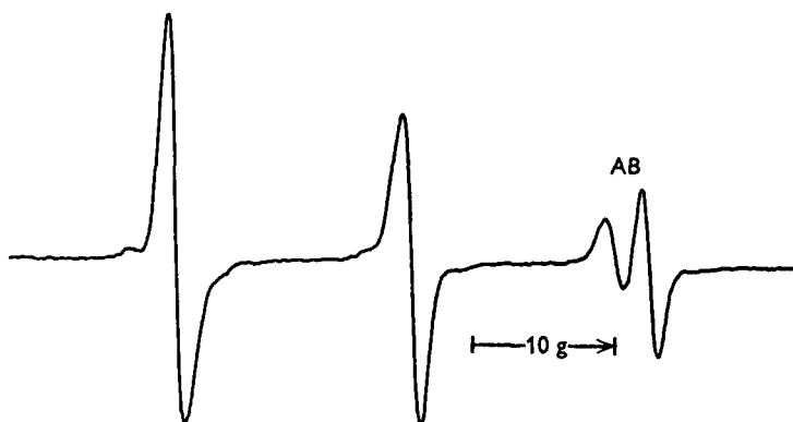
Fig. 10. The paramagnetic resonance of spin label V (see text) in the liquid-like hydrophobic region of the rabbit vagus nerve (A) and in the surrounding aqueous solution (B). The spin-label signals from these environments coincide for the other two hyperfine components of the spectrum.
