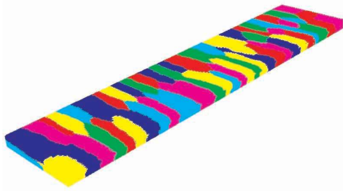
Figure 4.14: Mesh decomposed for 64 processors.
