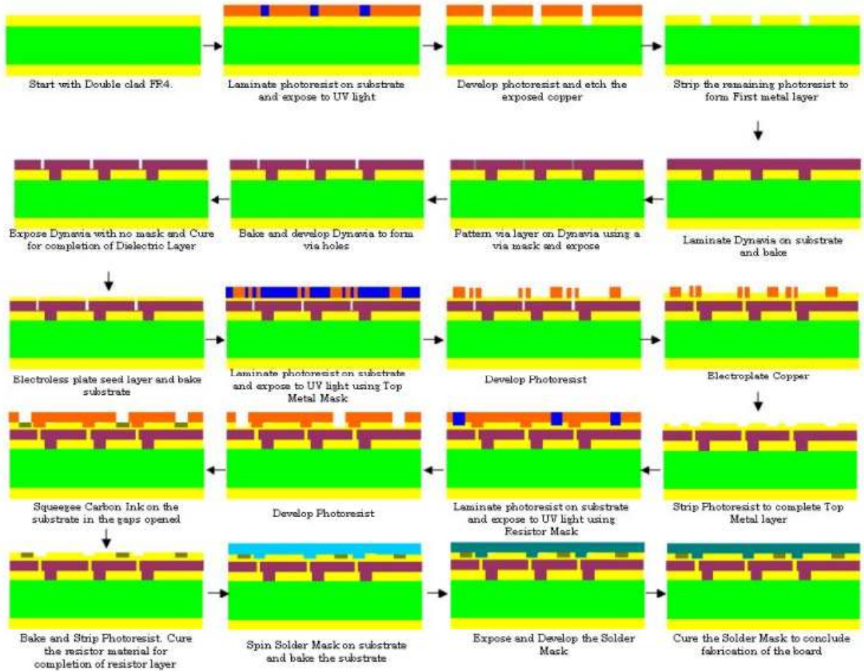
Figure 4.7. Fabrication process of passives
