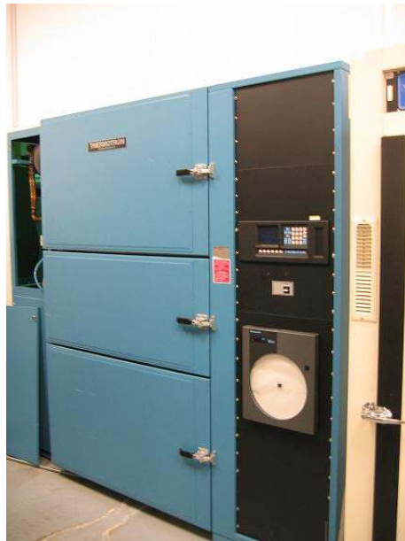
Figure 7.3. Picture of the Thermal Chamber used
