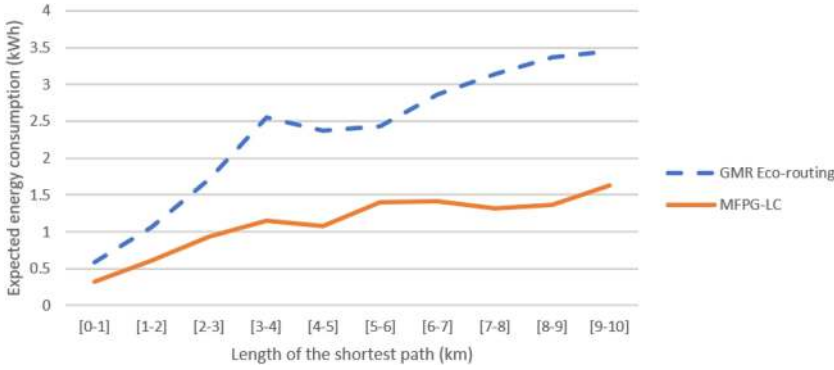
Fig. 15. The average EEC of the paths selected by the GMR Eco-routing method and the MFPG-LC method.
