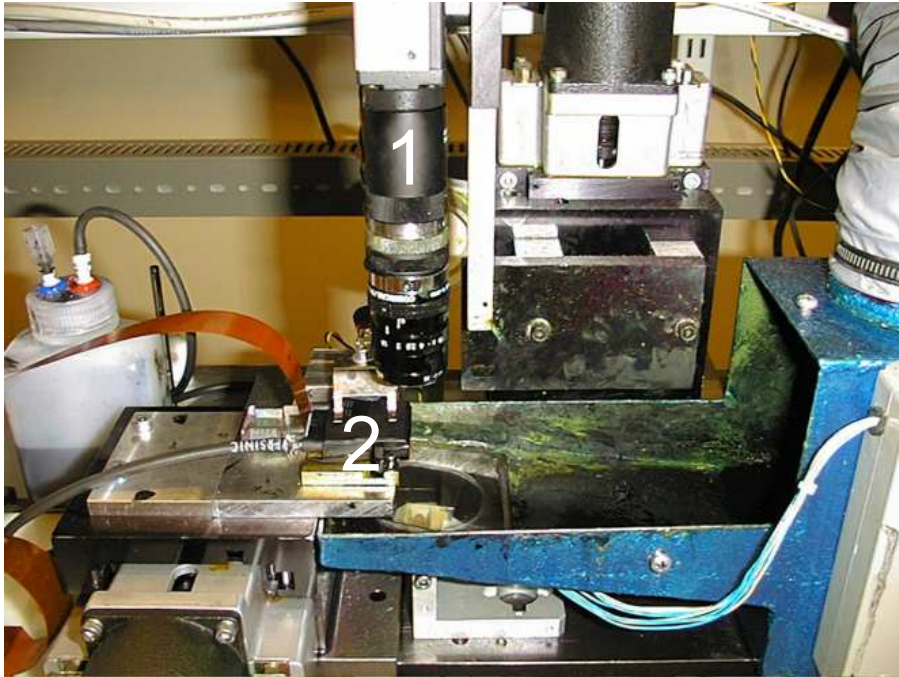
Figure 3.11. The stroboscope setup showing the CCD camera (1) and a mounted printhead (2).
