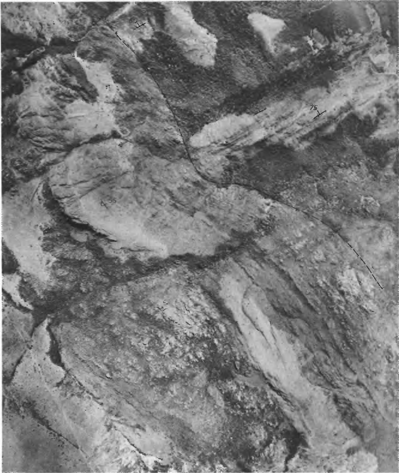
FIGURE 5.—Vertical aerial photograph showing the unconformity between the Minas Series (left) and the Rio das Velhas Series (right) in the Serra do Itabirito near N. 8,000, E. 3,000, Itabirito quadrangle. The Minas Series is here folded past the vertical and dips steeply east. The relief on the ancient pre-Minas erosion surface, formed on the hard quartzite in the Rio das Velhas Series, is somewhat exaggerated by the angle of view. Approximate scale, 1:10,000.
