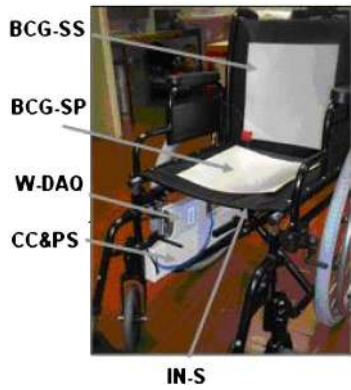
Fig. 1. Physiological parameters measurement system based on unobtrusive sensing units embedded on a wheelchair (W-DAQ module, CC&PS conditioning circuit, and power supply module, BCG-SP—ballistocardiography primary sensor, BCG-SS—ballistocardiography secondary sensor).
