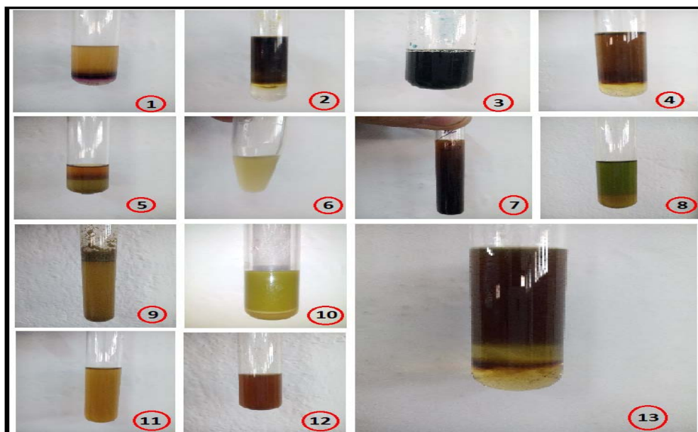
Fig. 1: Qualitative analysis of jute leaf extract, [1] Carbohydrate [2] Glycoside [3] Protein [4] Steroid [5] Cholesterol [6] Alkaloid [7] Phenol [8] Flavonoid [9] Saponin [10] Anthraquinone [11] Tannin [12] Phlobatannin [13] Terpenoid
