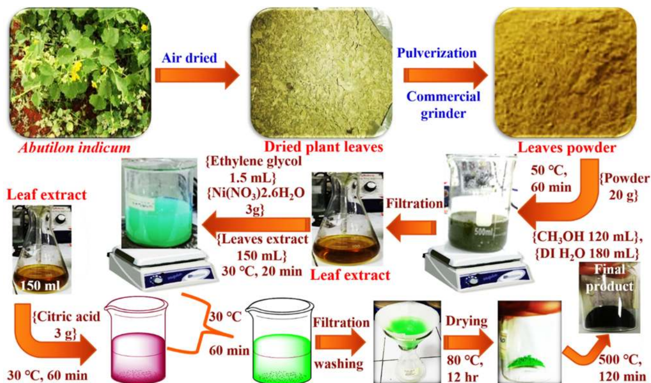
Figure 1 The scheme for the green synthesis of phytomolecules-coated NiO nanoparticles using Abutilon indicum leaves extract.
