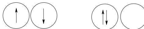
Figure 7. The outer orbitals of singlet oxygen. The opposite spin of the electrons in the outer orbitals makes the species energy-rich and highly reactive.
