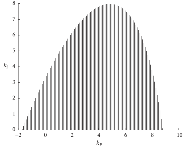
FIGURE 5: The stabilizing set of (k_p, k_i) values.
