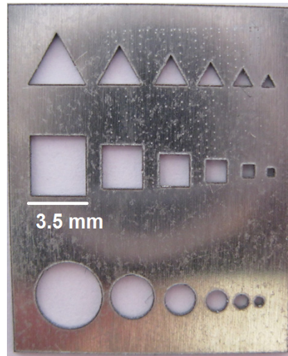
Fig. 12. Example of cutting through of the 0.3 mm thick aluminum sheet with the ns laser.
