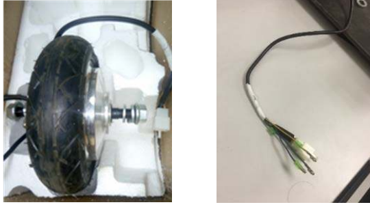
FIGURE 5. BLDC MOTOR WITH HALL SENSORS
