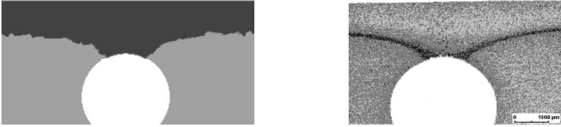
Figure 7: Influence of geometry on hardening profile. Simulation of electron hardening of a plate with hole parallel to the surface in 2 mm distance (left) in comparison with the corresponding experimental result (right), steel C45.
