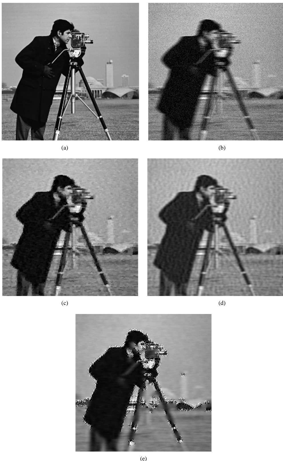
Fig. 1. Example of the LOMO LIM. (a) Original cameraman image. (b) Corrupted image ( 1 \times 9 uniform blur with \text{SNR} = 15 dB Gaussian noise). (c) Restoration using the LOMO-3 regularization operator. (d) Restoration using CLS. (e) Restoration using line process model.
