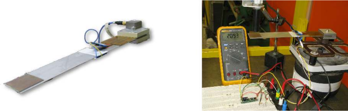
Figure 10. Piezoelectric harvester designed for traffic-induced vibrations (left), and view of the test set-up (right).
