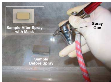
Figure 1. Set-up of sol-gel spray.
