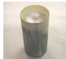
Figure 10. Thick BIT/PZT film deposited on a spherical concave surface.
