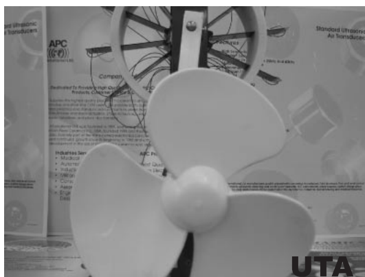
Fig. 1. Picture of the fabricated prototype “Piezoelectric Windmill”.
