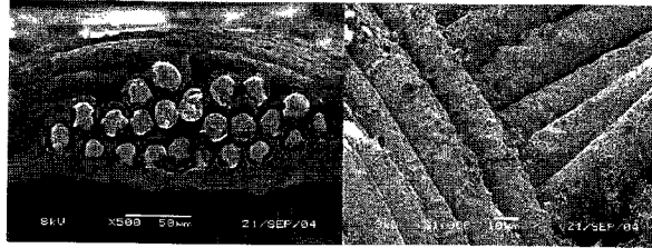
Figure 3. Cross section and top view of silver printed region of a Nylon fabric.
