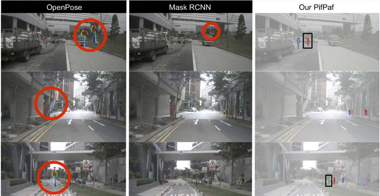
Figure 6: Illustration of our PifPaf method (right hand-side) against OpenPose [3] (first column) and Mask R-CNN [40] (second column) on the nuScenes dataset. We highlight with bounding boxes all humans that other methods did not detect, and with circles all false positives. Note that our method correctly estimates the waving pose (first row, first bounding box) of a person whereas the others fail to do so.
