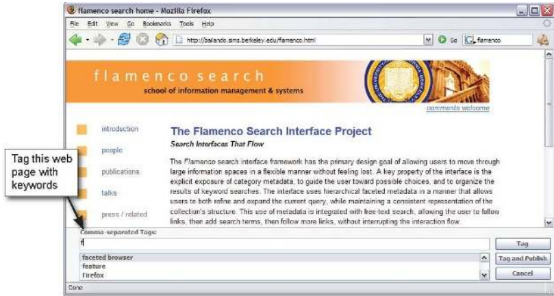
Fig. 3. Like del.icio.us, Piggy Bank allows each web page to be tagged with keywords. However, this same tagging mechanism also works for “pure” information items and is indiscriminate against levels of granularity of the information being tagged.
