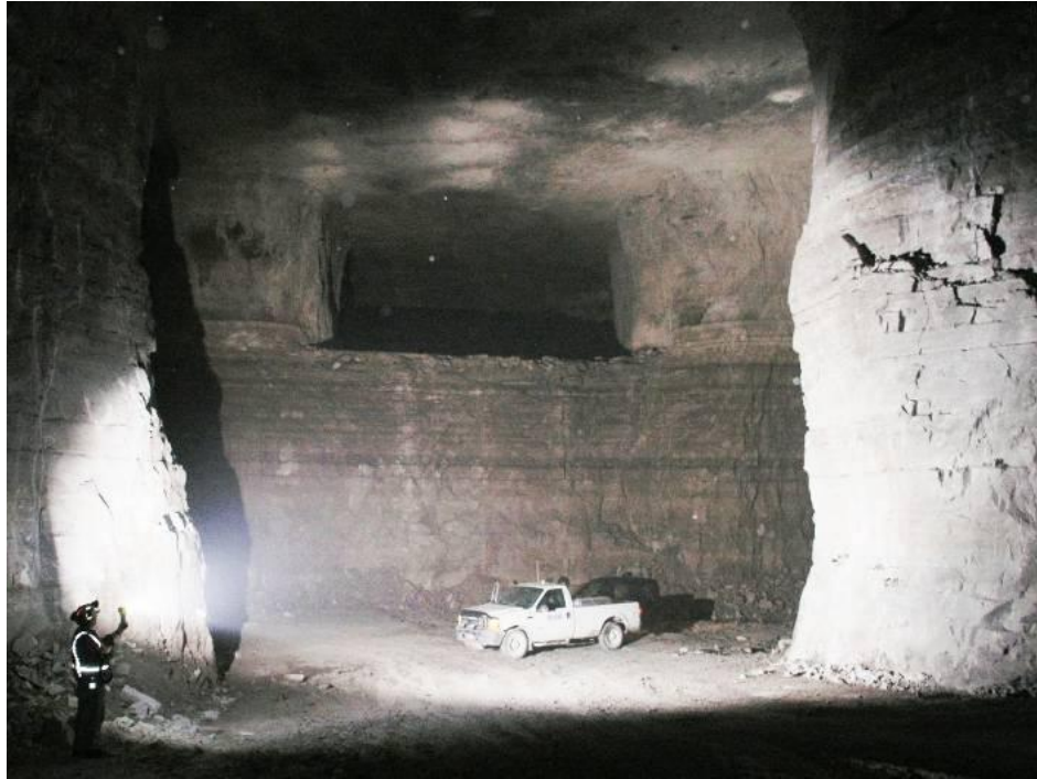
Figure 19. Example of bench mining of the floor between pillars in a limestone mine.
