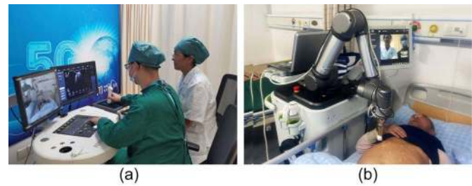
Fig. 2. Performance of robot-assisted teleultrasound based on the 5G network. (a) Doctors on the doctor side are manipulating a handheld controller, which can control the robotic arm. The duplicate control panel is used to adjust all the settings such as gain, depth, focus, and so on, as is performed on a real-ultrasound instrument. The screen is displaying ultrasonic images, and is monitoring the activities of the robotic arm and the probe. (b) Patient is receiving robotic lung ultrasound in the isolation ward, where there is no ultrasound specialist.
