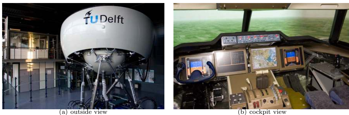
Figure 4. The SIMONA (Simulation, MOtion and NAvigation) Research Simulator (SRS) at Delft University of Technology, source: Joost Ellerbroek
