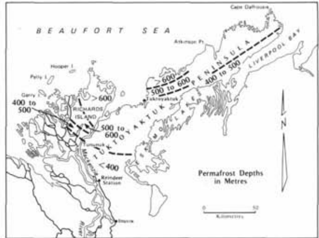
FIGURE 6. Permafrost depths based mainly upon geothermal data (JUDGE et al. , 1979; TAYLOR and JUDGE, 1977) and oil company drill hole records. The depth estimates are for undisturbed conditions
