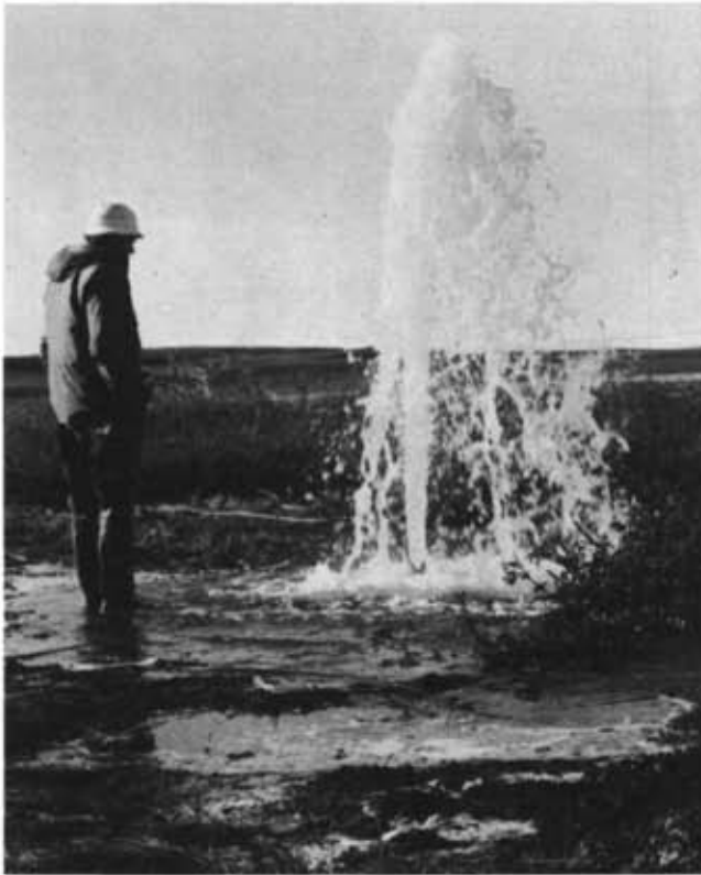
FIGURE 35. Drill hole flow from pingo 14. The water came from a depth of 22 m and jetted up 2.6 m high from a 7.5 cm diameter hole. The clear water was mineralized and cold. The orifice water temperature ranged from -0.05^{\circ}\text{C} to -0.10^{\circ}\text{C} .
