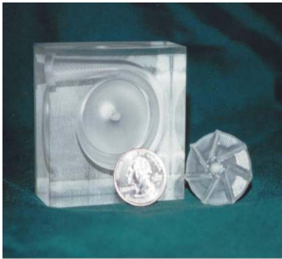
Figure 1.—Impeller and casing of acrylic model of blood pump
