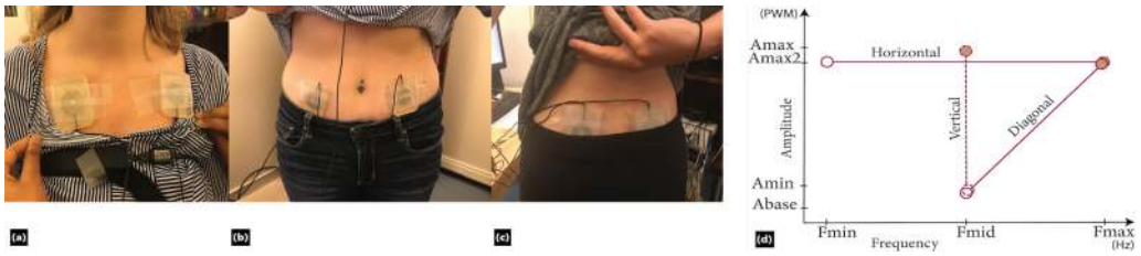
Fig. 3. C-2 factor chest placement (a); abdomen placement (b); lower back placement (c); frequency - amplitude representations of the three shapes (d).
