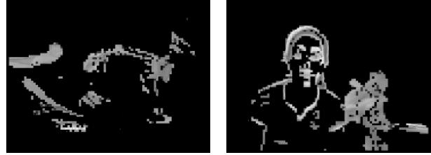
Figure 6. Dynamic pixels expressed by the wavelet coefficients in [Left] Movie #1 [Right] Movie #2. Graylevels indicate the temporal average of pixels values. Black regions represent static pixels.
