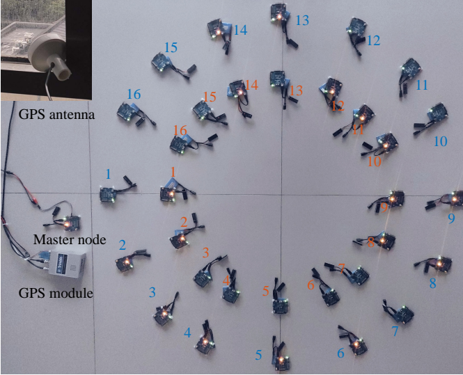
Fig. 6. Hardware testbed of a circular network by using Atmel SAM R21 wireless boards [28].
