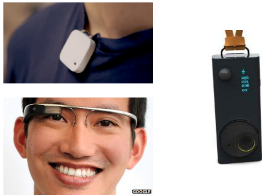
Fig. 1. Wearable camera devices. Clockwise from top left : Narrative Clip takes photos every 30 seconds; Autographer has a wide-angle camera and various sensors; Google Glass features a camera, heads-up display, and wireless connectivity. (Photos by Narrative, Gizmodo, and Google.)
