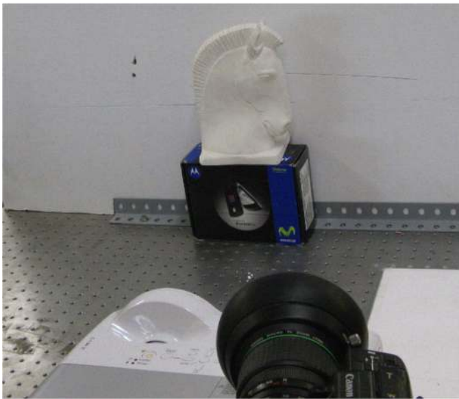
Fig. 8: Setup used for the camera-projector calibration and for the reconstruction of a 3D object.
