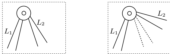
FIGURE 2. The initial position of the link L_2 (on the left) and an arbitrary position (on the right): the isometry representing the absolute position of L_2 on the right is the one taking it from its initial (dashed) position to the actual one.
