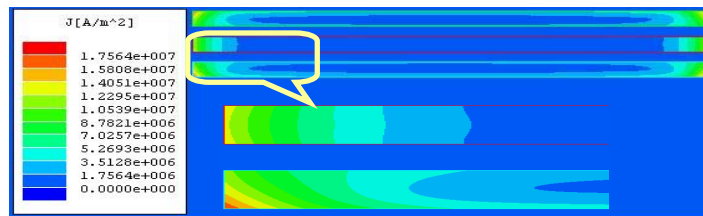
Figure 3.5 Proximity effect (three layers in parallel).
