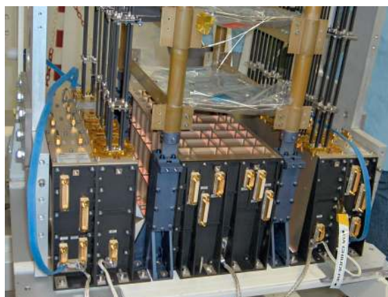
Fig. 19. Picture of the lower part of the LFI RAA during an advanced phase of the instrument flight-model integration showing the LFI back-end unit. The two lateral trays hosting the radiometer BEMs are symmetrically disposed to the left and right sides of the DAE-BEU box. The lower part of the straight stainless steel waveguides are shown.
