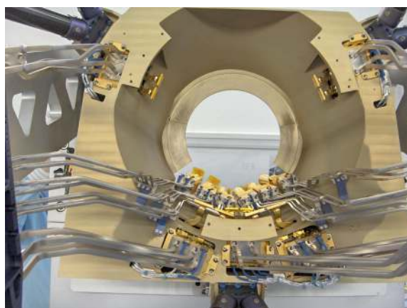
Fig. 18. Pictures of the LFI waveguides mounted on the RAA during the integration of the LFI flight model. Top : a view of the straight SS sections, black-painted on the outside and arranged in groups of four. On the upper part the Cu sections are connected through multiple flanges. The upper and lower mechanical support structures are also visible. The three interface levels corresponding to the three V-grooves are also shown. Bottom : back view of the LFI front-end unit showing the twisted Cu sections connecting to the FEMs. The waveguide routing and central hole in the main frame are designed to interface with the HFI front-end 4 K box.
