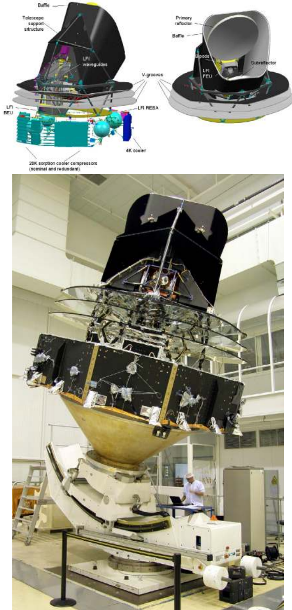
Fig. 5. Top: schematic of the Planck satellite showing the main interfaces with the LFI RAA on the spacecraft. Bottom: back view of Planck showing the RAA integrated on the PPLM. The LFI Back-end unit is the box below the lowest V-groove and resting on the top panel of the SVM.
