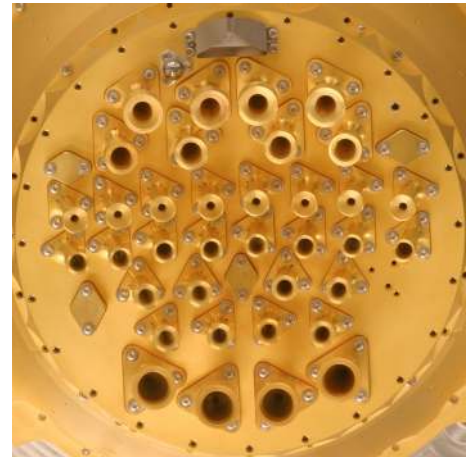
Fig. 4. Top: HFI focal plane layout. Empty circles represent the location of the front horn of each total intensity pixel. The crosses within the circles give the axis orientation of the dual-polarised detectors a and b of the PSBs. Bottom: top-view of the flight model 4 K focal plane array.
