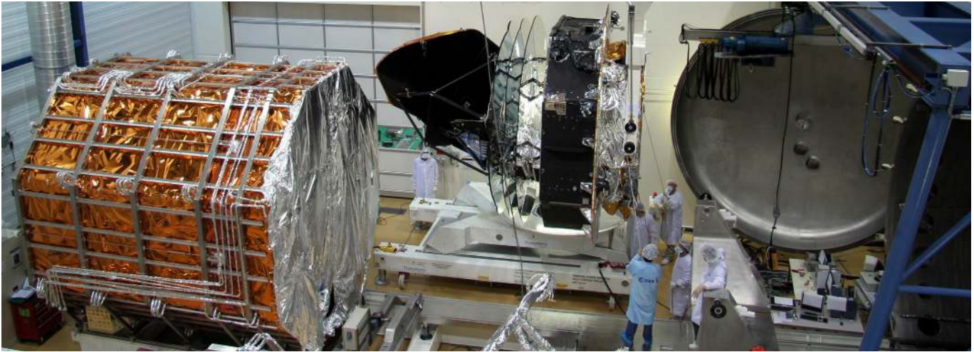
Fig. 9. Planck in configuration ready to enter into the CSL Focal 5 cryogenic simulator.
