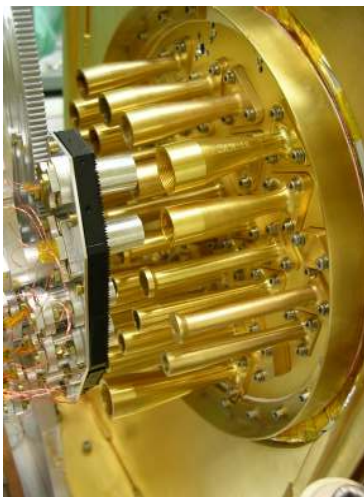
Fig. 7. Carbon fiber sources (OXT) in place in front of the HFI horns.
