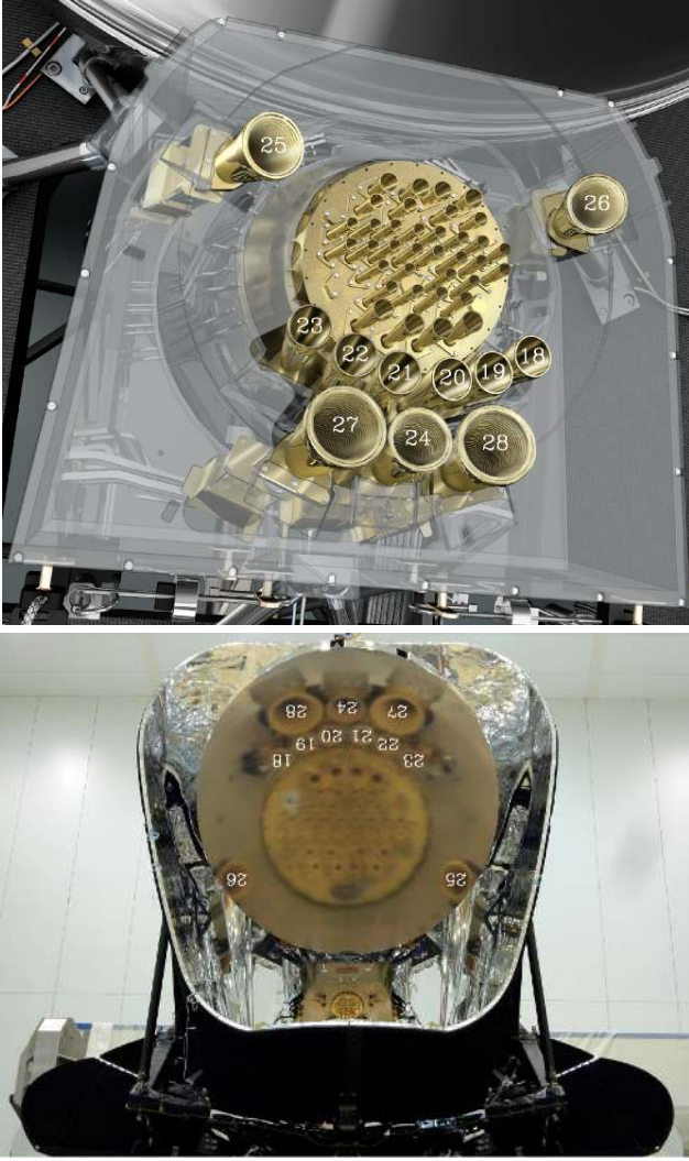
Fig. 2. A CAD model of the Planck focal plane, which is located directly below the telescope primary mirror. It comprises the HFI bolometric detector array (small feed horns on golden circular base) and the LFI radio receiver array (larger feed horns around the HFI). The box holding the feedhorns appears to be transparent in this view, to also show the elements inside and behind it ( top panel ). The HFI and LFI feed horns are seen reflected in the primary mirror of the Planck telescope in the clean room at Kourou, French Guiana ( bottom panel ). © ESA/Thales.
