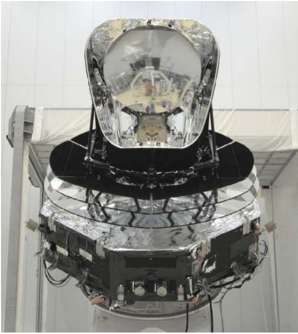
Fig. 1. The fully assembled Planck satellite a few days before integration into the Ariane 5 rocket. Herschel is visible by reflection on the primary reflector. Photo by A. Arts.
