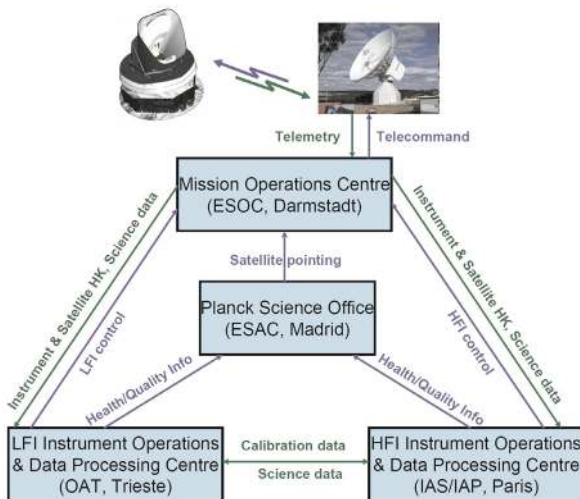
Fig. 16. A sketch of the centres involved in the Planck ground segment and the main data exchanges between them.
