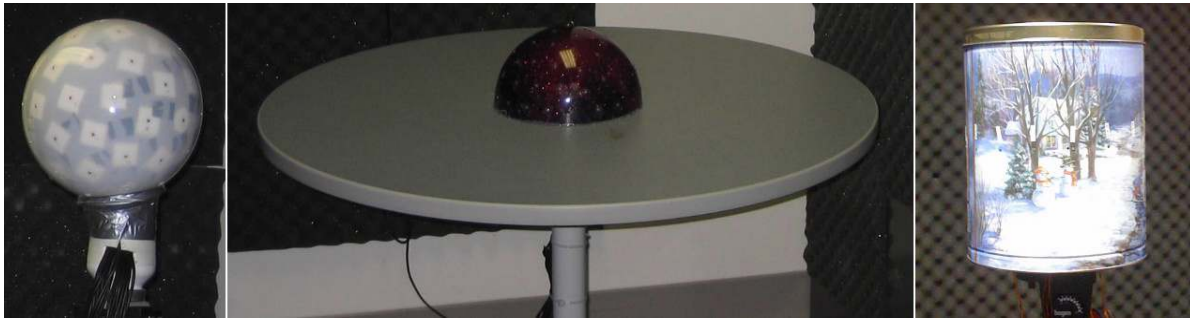
Fig. 1. Spherical (left), hemispherical (middle), and cylindrical (right) microphone arrays used. The hemispherical array is mounted on a circular table.
