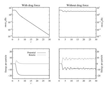
**Fig. 3.** 1D simulation of collapse of 1000 particles. With drag force the kinetic energy of the particles is efficiently dissipated and the particles collapse at subgrid scale towards infinite density. When the drag force is excluded the system cannot dissipate energy and a halo of particles, 10 grid cells wide, is formed.
