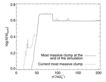
**Fig. 4.** Evolution of the most massive clump formed (solid line), which we traced back in time from the end of the simulation. It differs from the instantaneous most massive clump (dashed line) because the clumps have different feeding rate and can also experience mass loss, as in the episode that happened at  $\approx 90$  orbits (see text).
