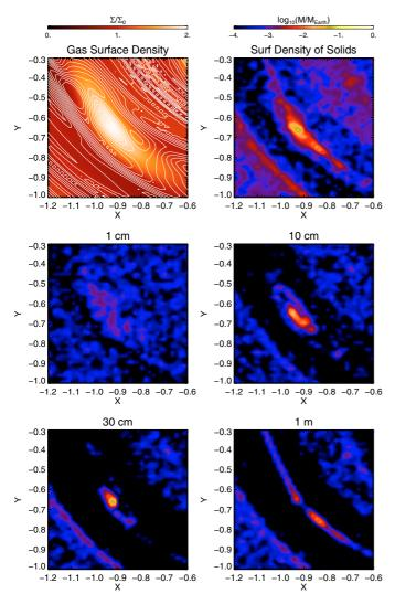
**Fig. 1.** Enlargement around one of the vortices in a snapshot at 20 orbits. Contours of |u| are superimposed on the gas surface density plot, showing that the density enhancement is associated with intense vorticity. In the *upper panel* we show the multiphase (total) surface density of solids, whereas in the *middle and lower panels* we show the contribution of each particle species. The vortical motion preferentially traps particles of  $a_{\bullet} = 10$  and 30 cm.
