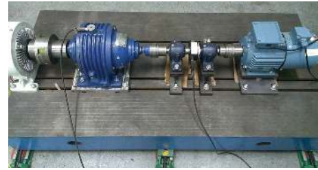
FIGURE 4: Test rig of a single-stage planetary gearbox.
