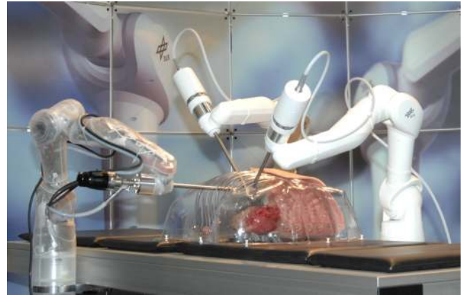
Fig. 1. The remote telemanipulator of the DLR system for minimal invasive robotic surgery, three versatile light-weight robots MIRO with 7 DoF and torque control, two surgical instruments with force-torque sensing attached to the white robot, a stereo endoscope carried by the transparent one.
