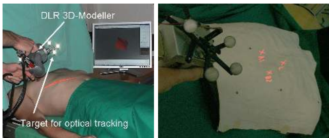
Fig. 11. Patient registration with the 3D-Modeller (left) and positioning with the AutoPointer (right).
