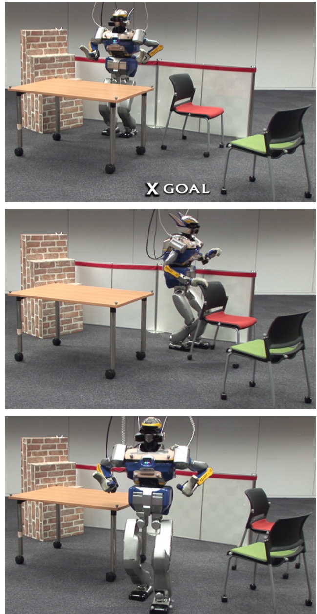
Fig. 1. Still frames from the autonomous planning and execution performed by HRP-2 ( time = 0s, 36s and 59s). The robot selects the chair for motion and performs the required walking and manipulation.
