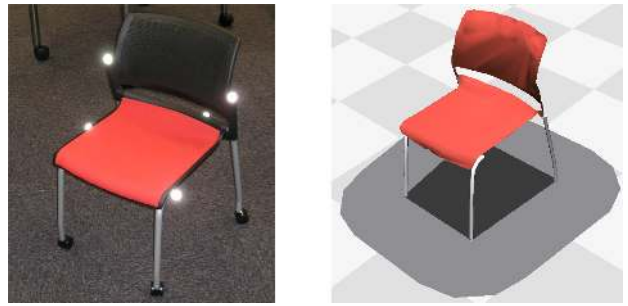
Fig. 3. (a) Chair used in our experiments with retro-reflective markers illuminated. (b) 3D model of the chair. The dark ground regions represent the planar obstacle and the C -space obstacle. The robot may walk on the grey region, but its torso COM must not enter it.
