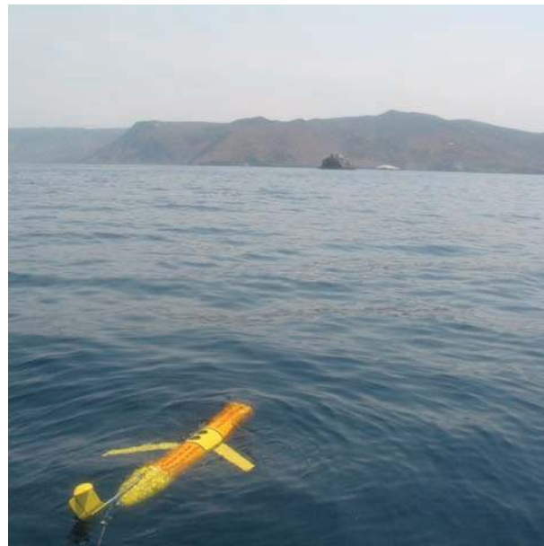
Fig. 2. One of the two Slocum gliders owned and operated by CINAPS. The glider has just been deployed and is preparing to start a mission. This picture was taken directly north of the entrance to Isthmus Cove off the northeast coast of Santa Catalina Island.
