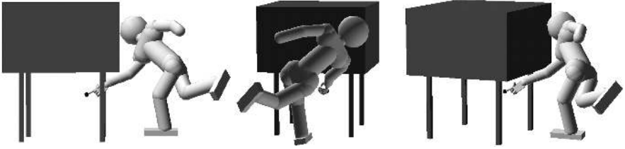
Fig. 3. Solution to a complex reaching movement under balance and collision constraints. The target for the right finger is illustrated as a black dot. Views from 3 different perspectives.
