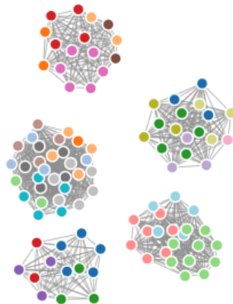
Figure 3: Example of a compatibility graph for a problem with 20 machines and 50 parts. Nodes of the same color belong to the same clique. The clusters correspond to different materials.
